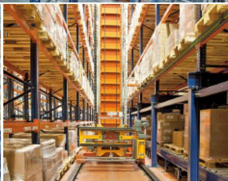
Integrated, trilateral extraction system with a rotating head that picks up and drops off pallets in three positions.
