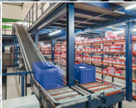
A wide variety of circuits can be configured, with straight sections, curves, inclines and even different levels.
