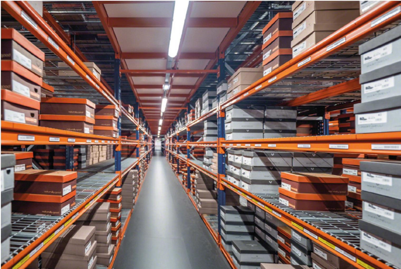
Longspan shelving is designed for warehouses where goods are deposited and removed manually from shelves. This system also makes optimal use of warehouse height, as the higher levels can be accessed mechanically by devices that lift the operator to the required height (stacker cranes or order picking forklifts) or via gangways located between shelves.
