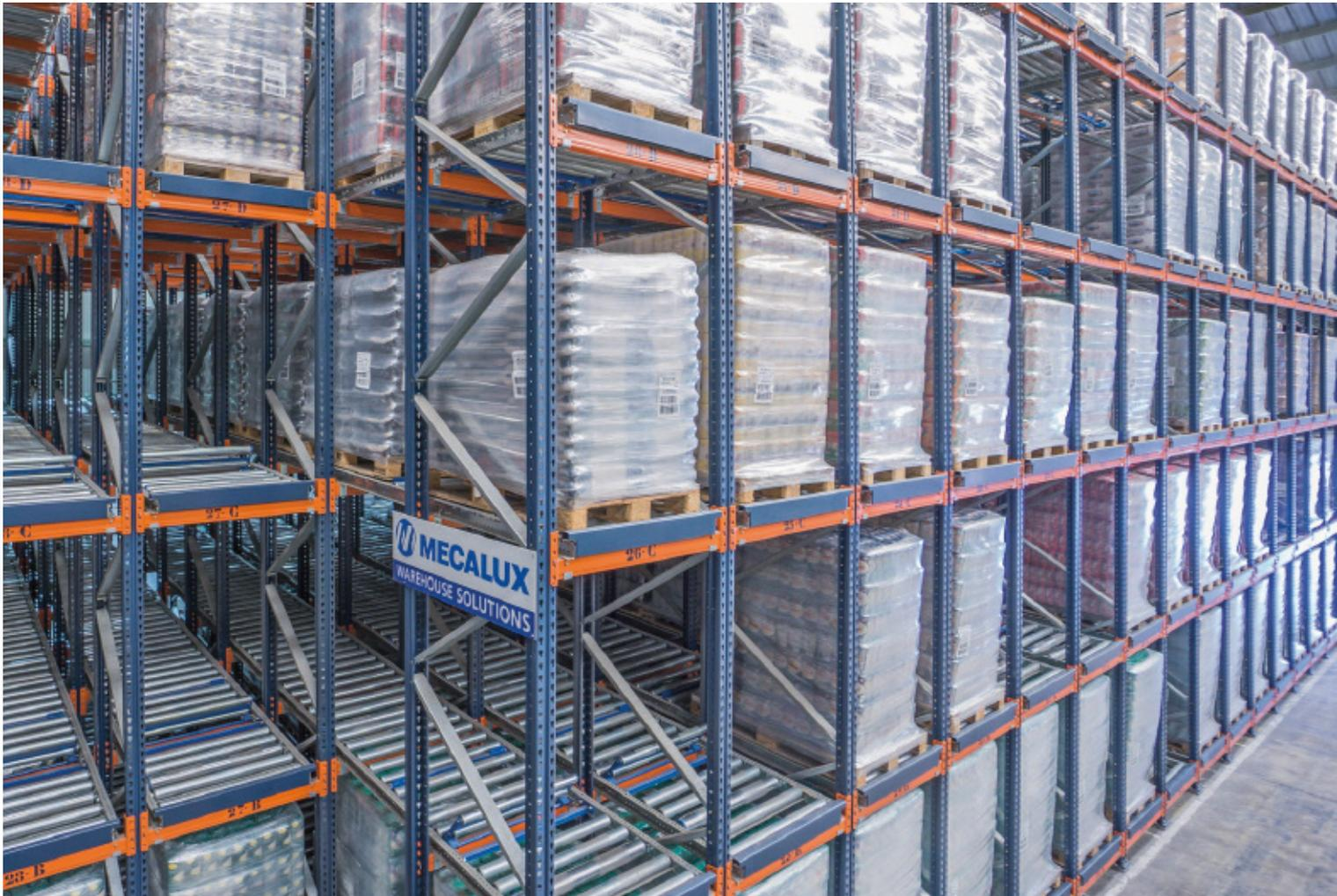
Live storage racking features roller tracks on a sloped lane to allow pallets to slide over them.
