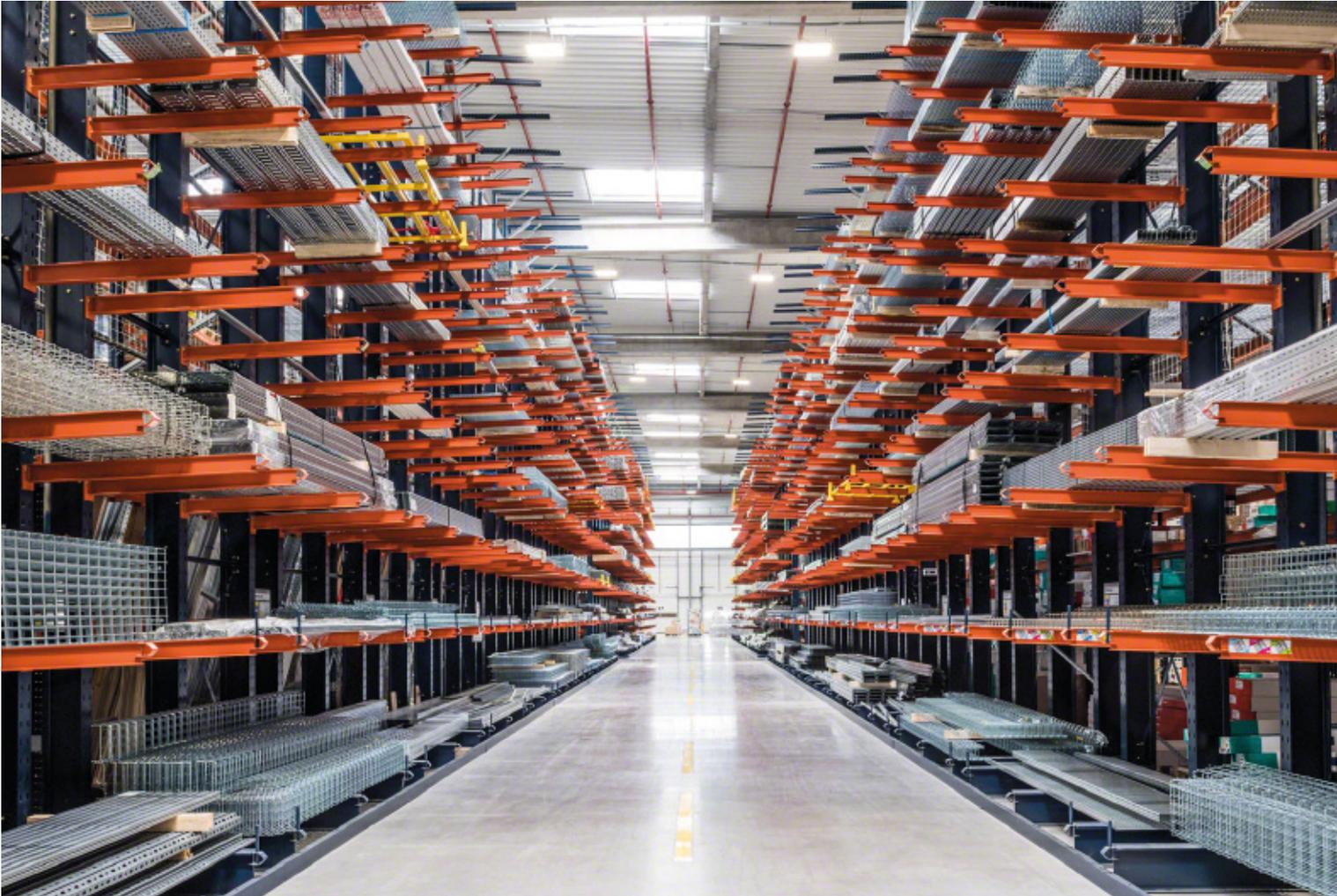
The system consists of columns with a vertical beam and one or two horizontal beams at the base to provide stability. A series of arms are attached, onto which the load is placed.
