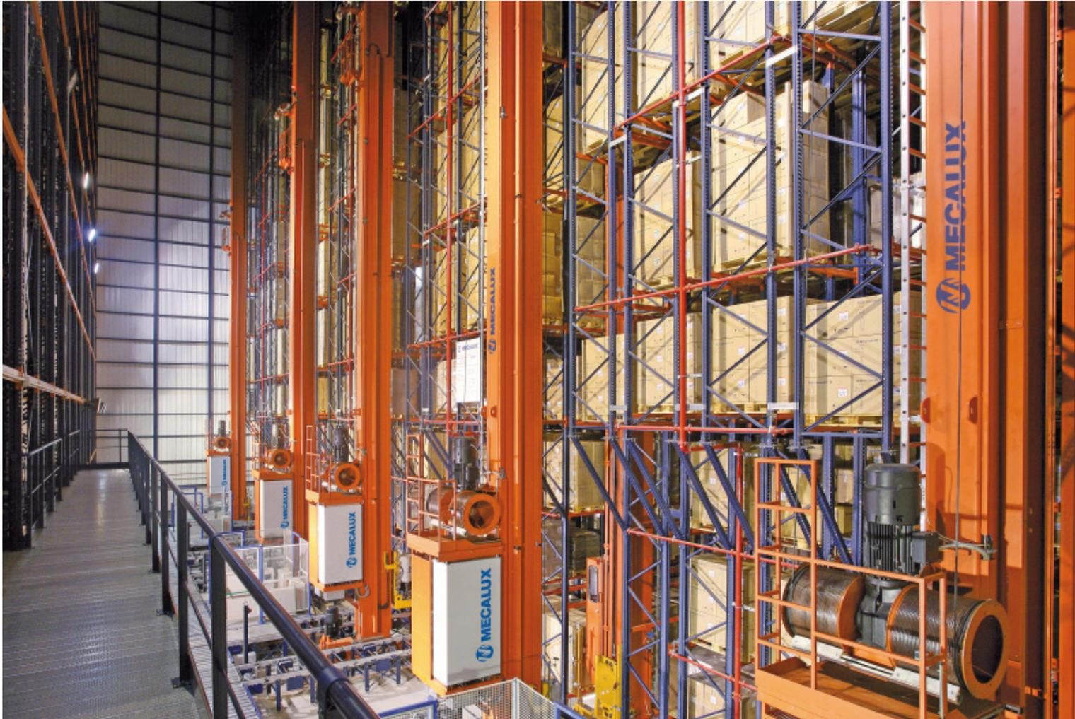
Stacker cranes are machines designed for the automated storage of materials by means of automatic mechanical movements. Materials are inserted and extracted at the same time (known as a combined cycle). This increases the productivity of the installation and also reduces the resources required for it to function.
