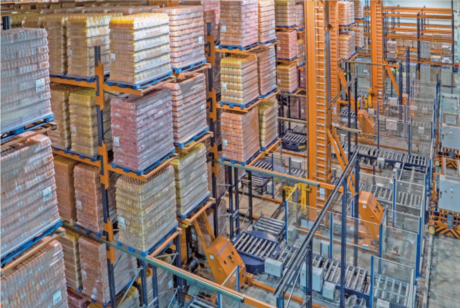
Automatic trilateral stacker cranes make it very easy to automate warehouses with conventional racks where a manually operated lift truck is used, both in pre-existing warehouses and in new facilities.
