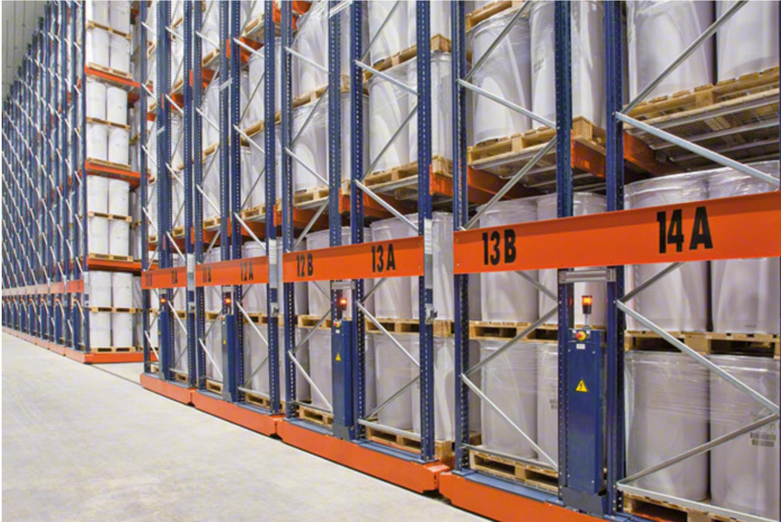
The racking is mounted on mobile bases which move along rails, eliminating the need for multiple access aisles and increasing storage capacity.
