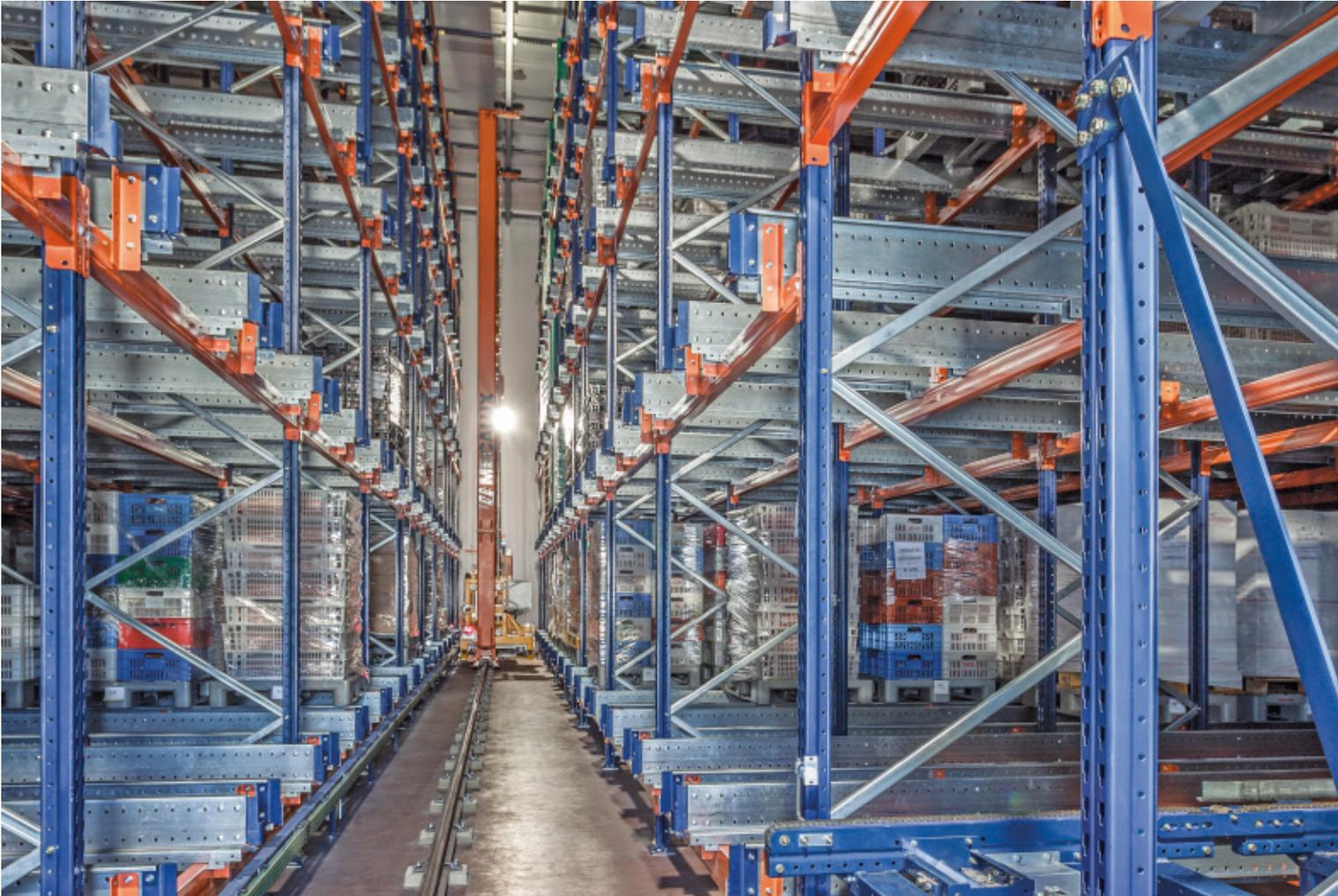
This system involves the incorporation of automated equipment in the handling processes of high-density warehouses. As a result, the forklifts are replaced by stacker cranes or transfer cars carrying the Pallet Shuttle and the load in their cradle.
