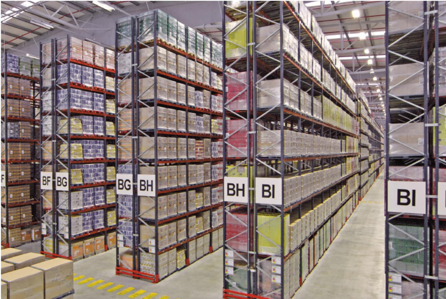
Conventional pallet racking is the best solution for warehouses where it is necessary to store a wide range of articles on pallets.
