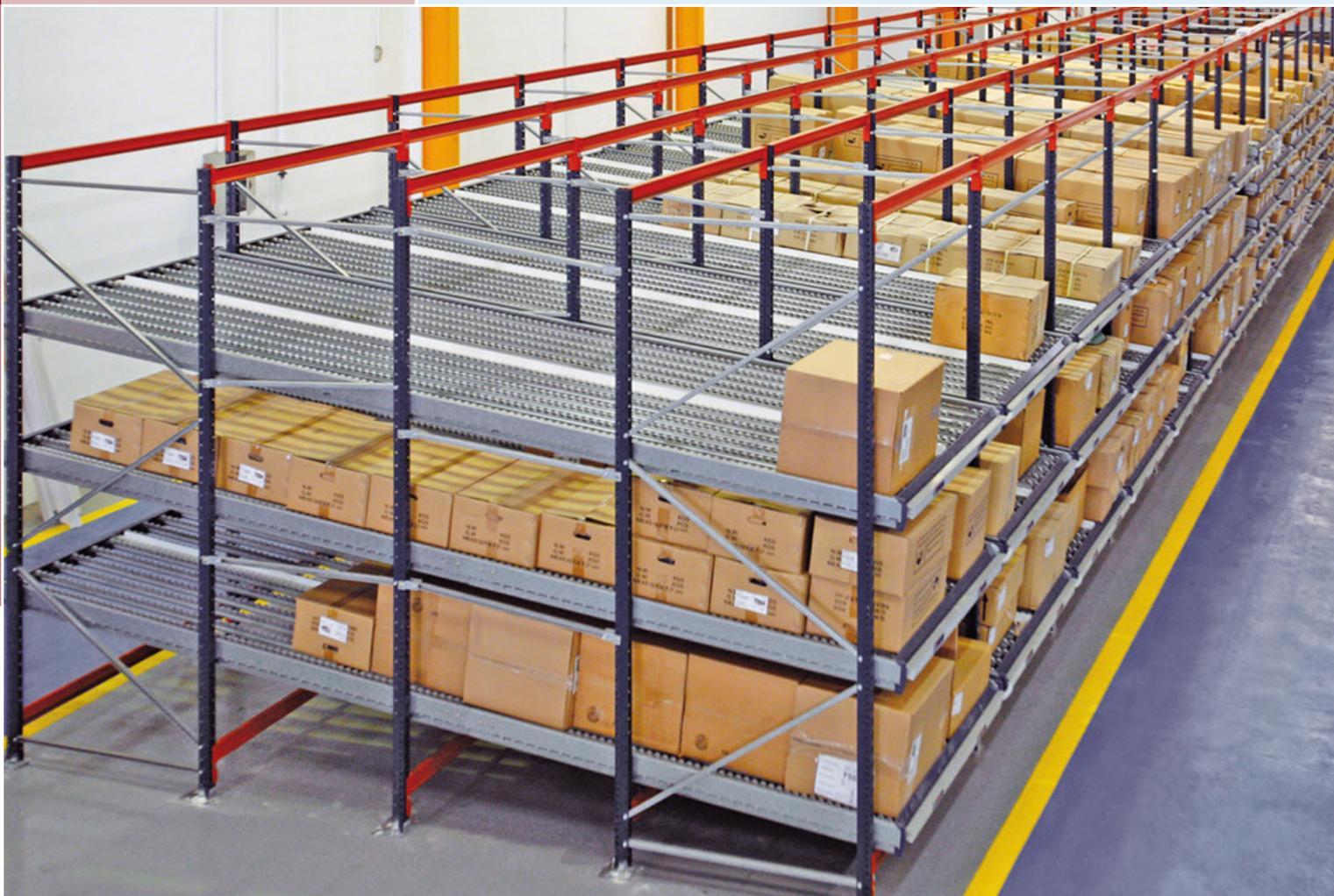
Live storage for picking. Goods are placed onto sloped roller tracks where they then roll at a controlled speed towards the lane exit by the force of gravity.
