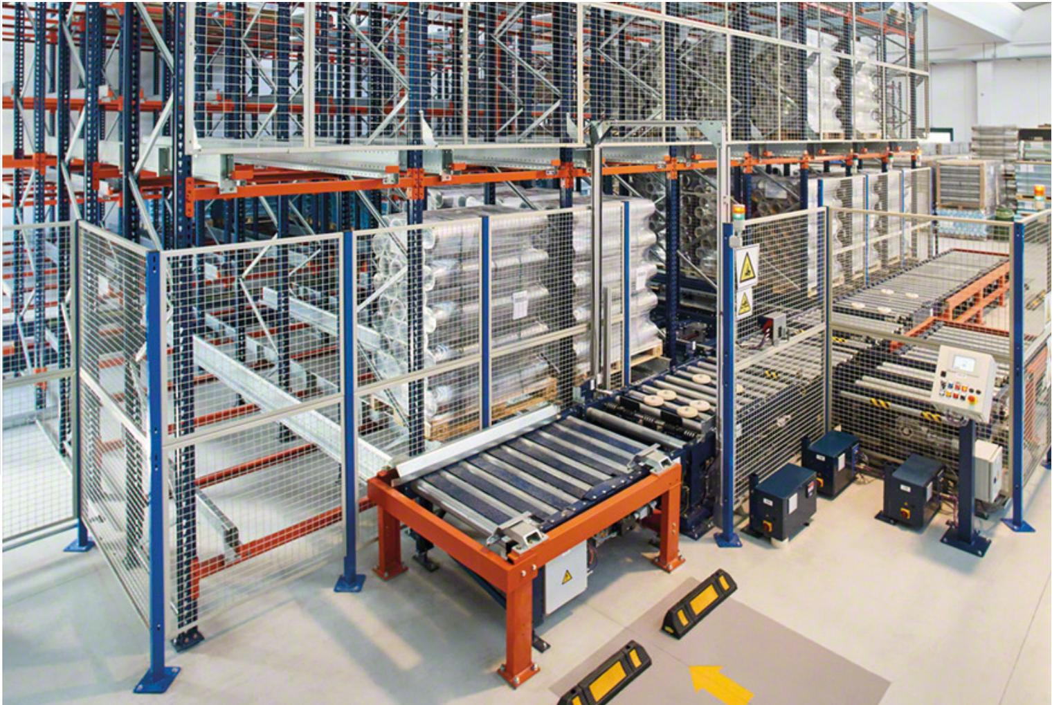
These create a protected space in work areas where there is automated equipment and robotics. They also keep the area free of possible materials shed by the action of machines.
