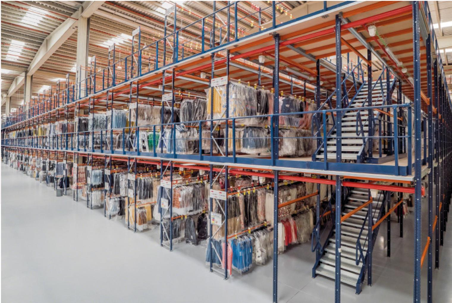
The full use of the warehouse's height is enabled, installing high racks with one or more gangway levels supported by the racks themselves.
