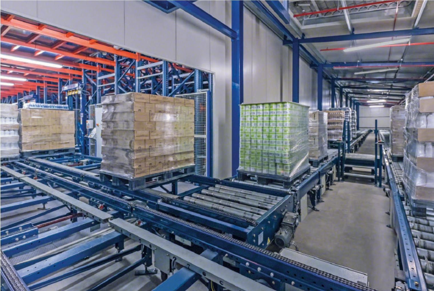
Conveyor systems represent an ideal combination between the efficiency of the stacker cranes and the entry, dispatch and handling processes of the load units. Logistics operations require a continuous flow of materials, as pallets and/or boxes must be taken from a storage or production location or from an overflow warehouse to dispatch or production areas.
