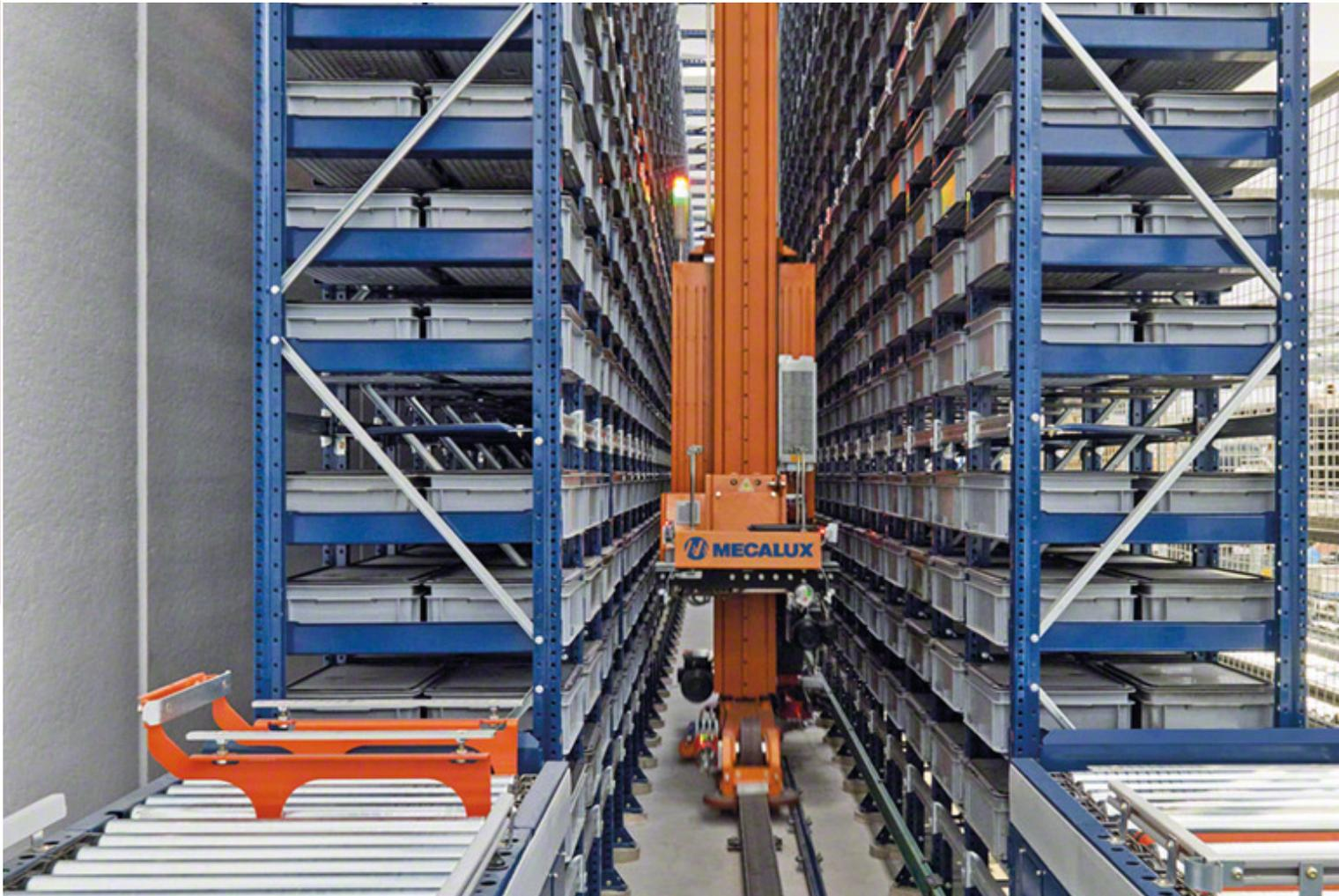
Stacker cranes for boxes are designed to achieve a high level of productivity and manage loads with boxes or trays.
