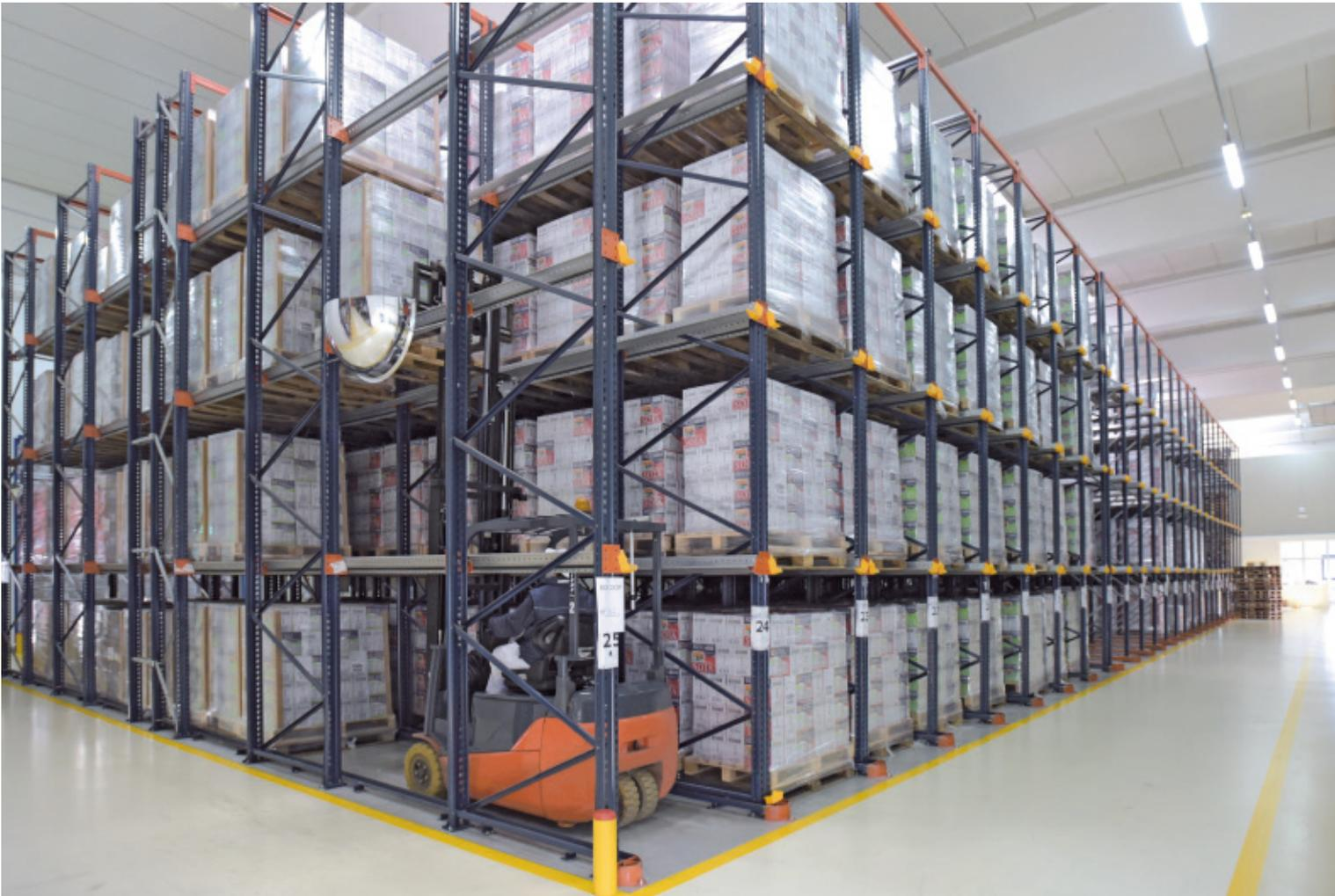
This storage concept consists of a set of racking units which form an internal lane with support rails for the pallets. The forklift enters the lane with the load elevated above the support rail that it will be placed upon.
