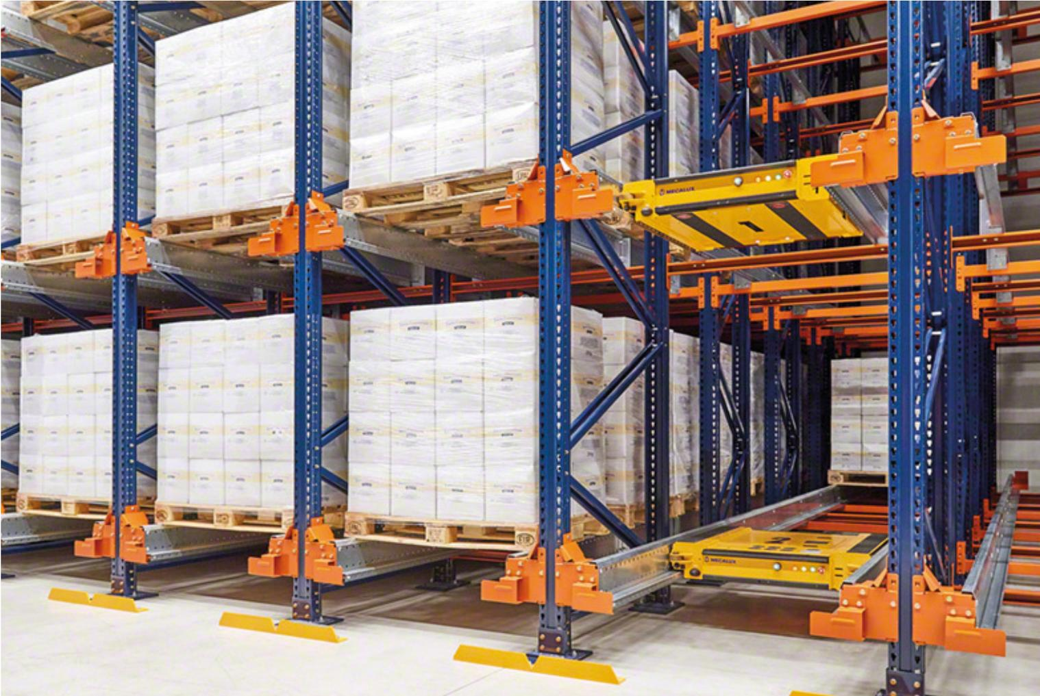
This is a high-density pallet storage system which facilitates the independent loading and unloading of goods from an electric shuttle called a Pallet Shuttle, eliminating the need for forklifts to enter the racking.
